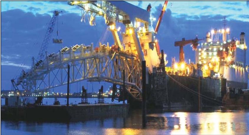
The Solitaire in Rotterdam harbour can lay pipes for oil and gas in oceans to depths over 2700 m using the S-lay method over its stinger. This floating factory ship with a length of 300 m (excluding stinger) accommodates 420 men. (Photo: Dirkjan Ambtman).
